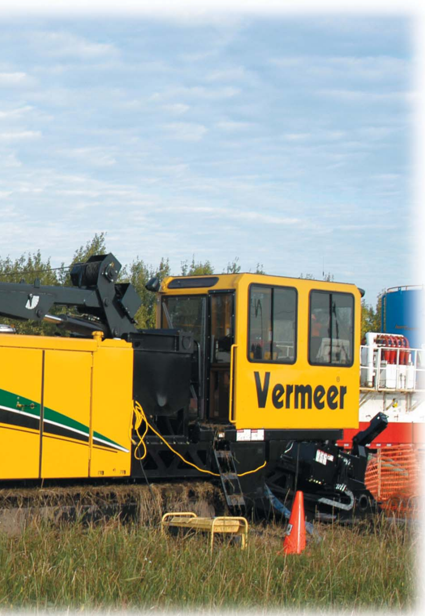
50,000 ft/lbs of torque High torque for drilling in difficult ground formations and turning large back reamers.
